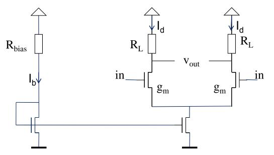
Current efficiency,  $\eta_1 = 2I_d/(I_b + 2I_d)$ . Note,  $I_b$  may need to be large for eg. low noise
