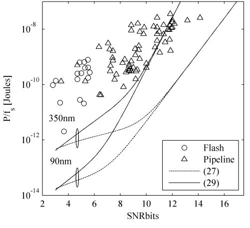
Plot of minimum ADC power for two processes
