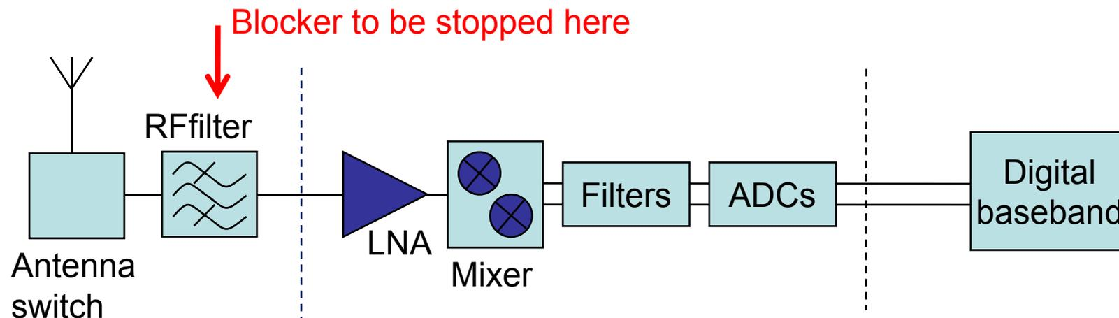
Need narrow band passive RF filters at input.
