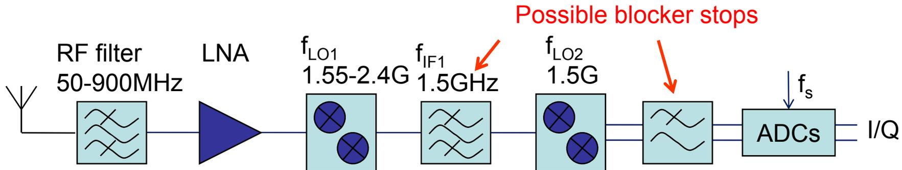
1dBm blocker at ADC: We can choose  $f_s=100\text{MHz}$  gives  $n=16$  (commercially available, eg. 160MS/s 16b 1.45W).
