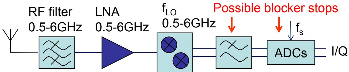
Gain to be supplied by low-pass filter or ADC
