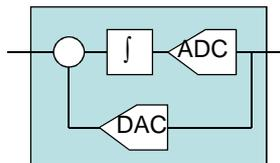
Utilizing a 1st order  $\Sigma\Delta$ -loop in ADC
