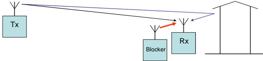
**Weak signal from Tx in presence of strong disturber (blocker)**
