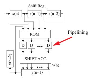
A set of D flip-flops has been placed between the ROM and the shift-accumulator to allow the two operations to overlap in time, i.e., the two operations are pipelined.
