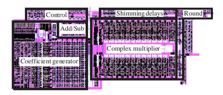
The maximal clock frequency at 3 V supply voltage is 133 MHz with a power consumption of 30 mW (excluding the power consumed by the clock).
