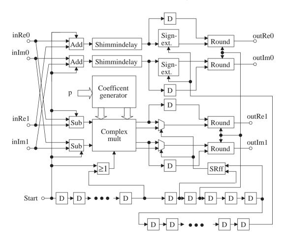
The decimation-in-frequency radix-2 bit-serial butterfly PE has been implemented in a 0.8 µm standard CMOS process.
