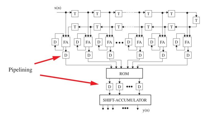
The logic circuitry has been pipelined by introducing D flip-flops between the adders (subtractors) and the ROM, and between the ROM and the shift-accumulator.
