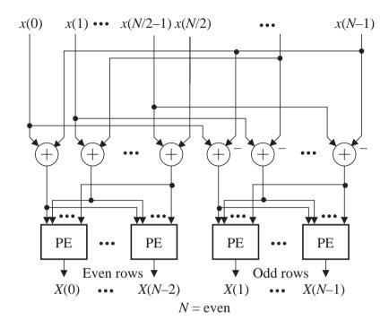
A 2-D DCT for  $16 \times 16$  pixels can be built using only one 1-D DCT PE which itself consists of 16 distributed arithmetic units with N = 8.
