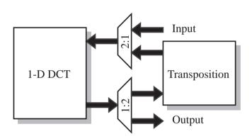
In the second phase, the columns in the intermediate array are successively computed by the processing element.
