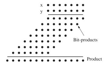
In a *tree-based multiplier* the bit-products are often added using full-adders.
