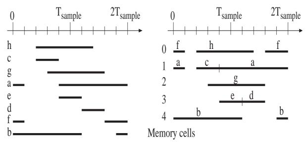
c) Each variable requires read and write within 2 sampling periods, i.e., total 16 memory accesses are needed.  $T_{access} = \frac{2}{15 \times 10^6 \times 16} = 8.3 \text{ ns.}$
