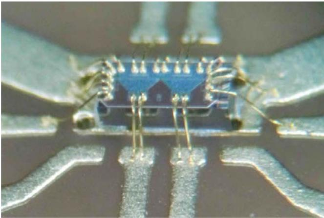
Differential PA,  $V_{dd}=3$  V,  $f=2412$  MHz
