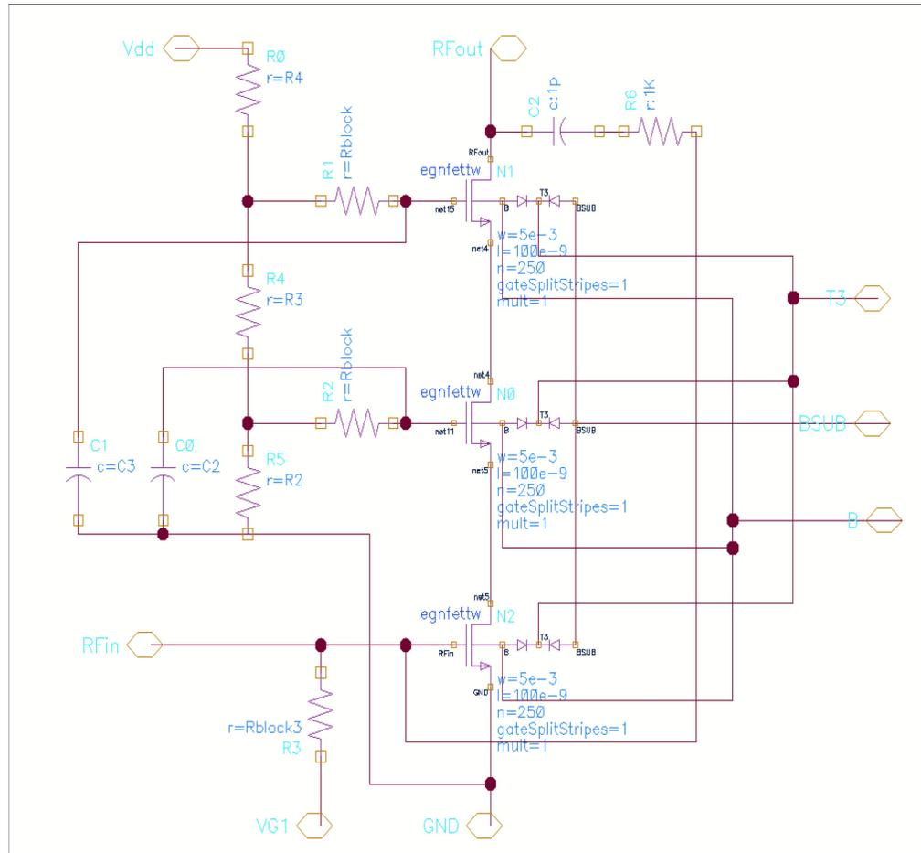
$W = 6000 \text{ } \mu\text{m}$  ( $10 \text{ } \mu\text{m} * 10 * 60 \text{ cells}$ )
