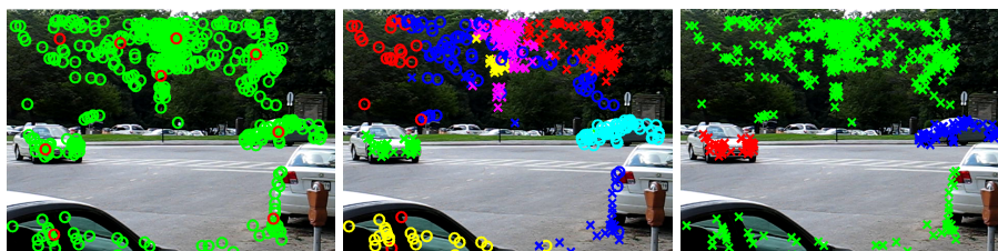
Fig. 1. A K-means initialisation example on the left. On the centre the classification result before the merging, and the final merged results on the left.
