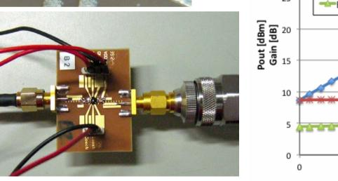
Differential PA, Vdd=3 V, f=2412 MHz **P-1dB = 32,5 dBm** (1,8 W). Class AB, efficiency over 50 % for unmodulated signal.
