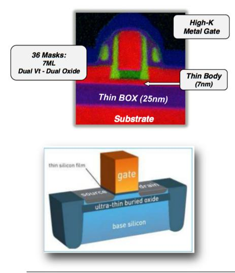
L<sub>g</sub>=24 nm, T<sub>ox</sub>=1.8 nm, V<sub>sup</sub>=1.0 V ultra-thin silicon: 7 nm ultra-thin buried oxide: 25 nm
