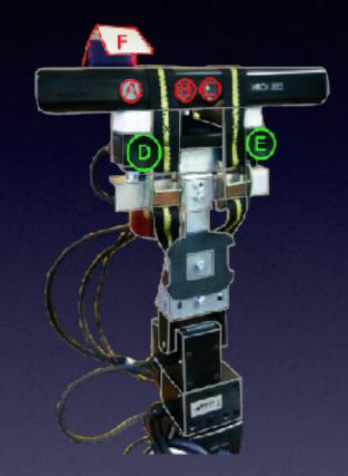
A: SLP projector (unused) B: RGB camera (unused) C: NIR camera (unused) D: Right wide-angle camera E: Left wide-angle camera F: SLP diffusor (unused)
