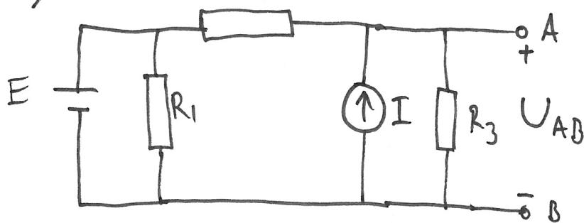
$$\begin{aligned} E &= 4.0 \text{ V} \\ I &= 3.0 \text{ A} \\ R_1 &= 4.0 \Omega \\ R_2 &= 5.0 \Omega \\ R_3 &= 2.0 \Omega \end{aligned}$$
