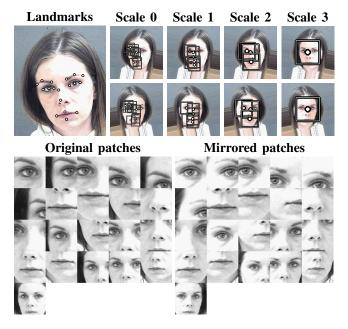
Figure 1: Facial landmarks and image patches used. Example from MORPH-II dataset (female, age 25). Top left: Original image with facial landmark points. Top right: extracted image patches and corresponding scale levels, original orientation (first row) and mirrored (second row). Bottom: resulting greyscale patches, original orientation (left) and mirrored (right). Artifacts at image borders are due to border replication in the rectification step.
