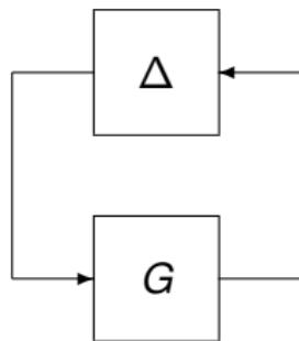
If  $G$  is stable and  $\|G\| < 1$  then the closed loop system is stable if  $\|\Delta\| \leq 1$ .
