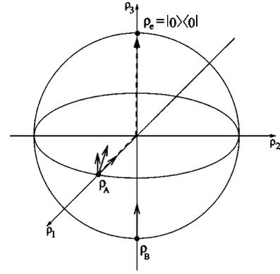
FIG. 4. Solid arrow: dissipation operator in two different states (in  $\rho_A$  it is decomposed into radial and tangential components) for the two-level spontaneous emission model. Dashed line: possible “controlled” trajectory.
