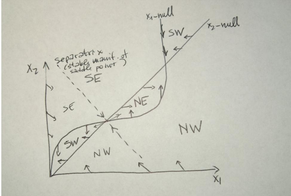
Figure 14: Nonlinear phase plane analysis in 2D for positive autoregulation with Hill kinetics.
