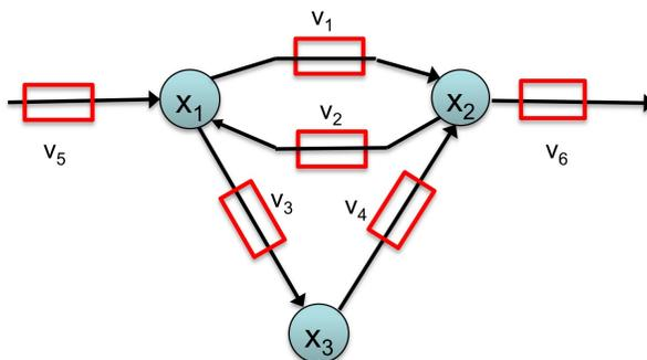
Figure 7: Example of reaction network with (unfeasible) loop.
