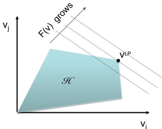
Figure 10: The level surfaces of the linear cost function  $F(v)$  on the polytope  $\mathcal{H}$  of admissible fluxes. The LP problem (4) has a unique solution  $v^{\text{LP}}$ .
