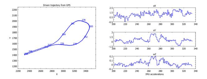
GPS gives good position. IMU gives accurate accelerations. Combine these to get even better position, velocity and acceleration.
