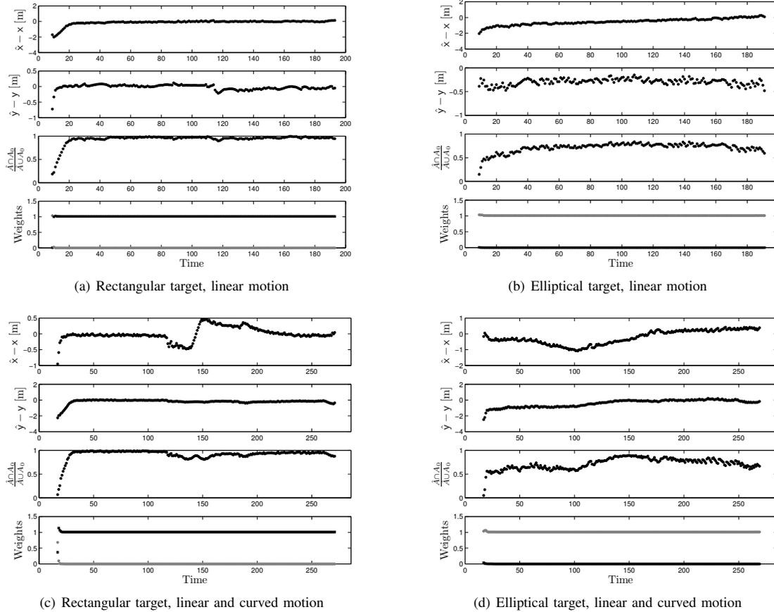
Figure 5. Simulation results: the top row shows linear motion (Figure 6(a)), the bottom row linear and curved motion (Figure 6(b)). Each figure shows the estimation error in  $x$  and  $y$  position, the IOU measure and the sum of the weights for each target type (black is rectangles, gray is ellipses).
