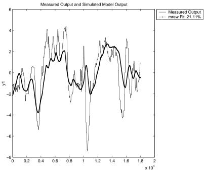
Dashed line:  $\kappa$ -number after the vessel, actual measurements. Solid line: Simulated  $\kappa$ -number using the input only and a process model estimated using the first 200 data points.  $G(s) = \frac{0.818}{1+676s}e^{-480s}$
