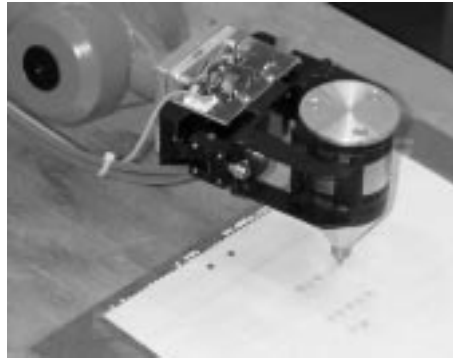
Figure 9.4 A possible configuration of the accelerometer on the IRB1400.
