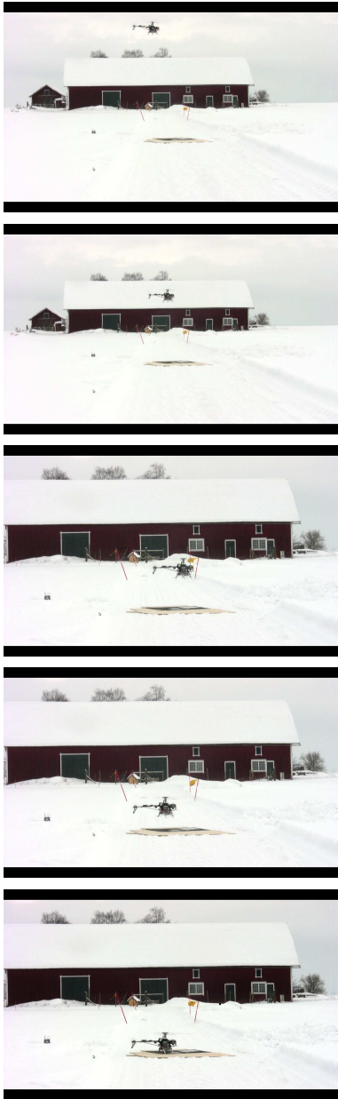
Fig. 9. Sequence illustrating an autonomous helicopter landing. In the top photograph, the UAV has just arrived, using the assisted mode, at a GPS position roughly 5 m above the landing platform. Here, the landing mode is activated and the UAV lands autonomously, relying on the camera and the vision system for measurements.
