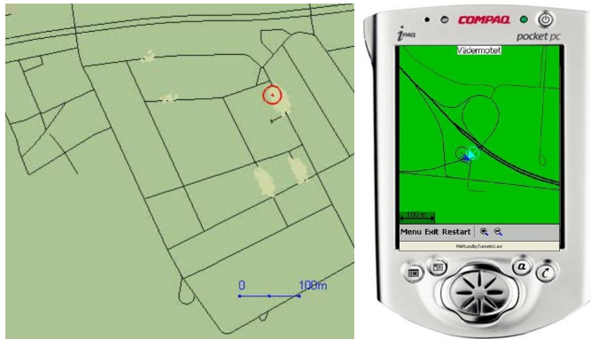
Figure 3: Left: Example of multimodal posterior represented by a number of distinct particle clouds from NIRA Dynamics navigation system. This is caused by the regular road pattern and will be resolved after a sufficiently long sequence of turns. Right: PF in an embedded navigation solution run in real-time on a pocket PC.
