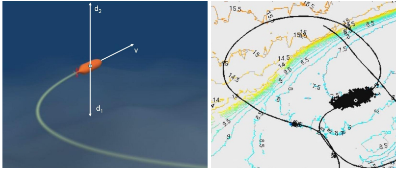
Figure 1: The left plot is an illustration of an underwater vessel measuring distance d_1 to sea bottom, and absolute depth d_2 . The sum d = d_1 + d_2 is compared to a bottom map as illustrated with the contours in the plot to the right. The particle cloud illustrates a snapshot of the PF from a known validation trajectory.
