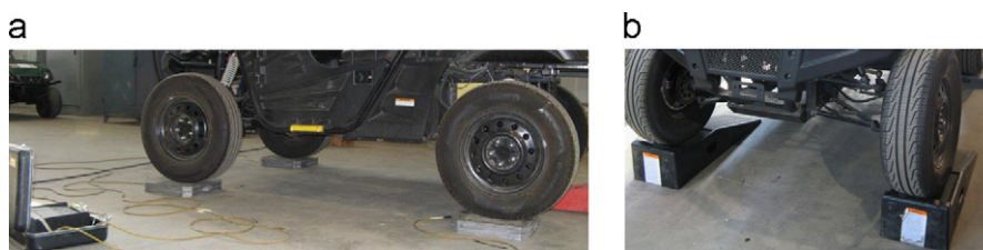
Fig. 4. Normal force measurement: (a) on flat ground and (b) front wheels lifted.
