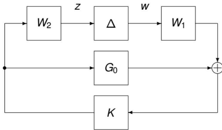
For which uncertainties,  $\Delta$ , is the closed loop system stable. The nominal system with  $\Delta = 0$  is assumed to be stable.
