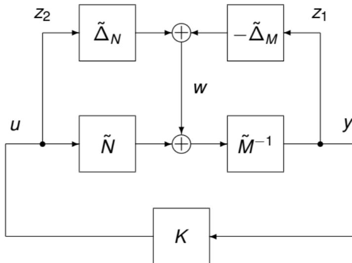
The transfer function from  $w$  to  $\begin{bmatrix} z_1 \\ z_2 \end{bmatrix}$ :
