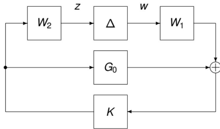
The transfer function from  $w$  to  $z$ :  $W_2 K \underbrace{(I - G_0 K)^{-1}}_{S_0} W_1 = W_2 K S_0 W_1$
