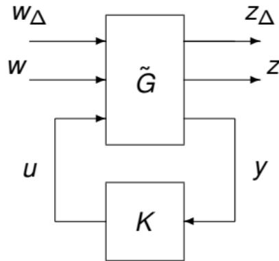
Minimize  $H_\infty$ -gain from  $\begin{bmatrix} w_\Delta \\ w \end{bmatrix}$  to  $\begin{bmatrix} z_\Delta \\ z \end{bmatrix}$ .
