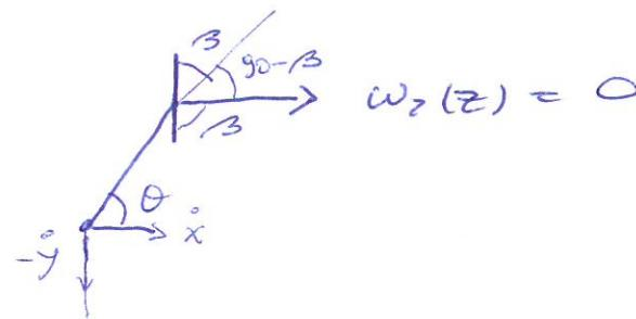
$$\begin{aligned} & \dot{x} \sin(\theta + \beta) \\ & - \dot{y} \cos(\theta + \beta) \\ & - L \cos \beta \dot{\phi} = 0 \end{aligned}$$
