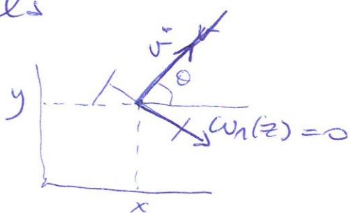
$$\begin{aligned} \omega_n(z) &= \dot{x} \cos(90-\theta) - \dot{y} \cos \theta = 0 \\ &= \dot{x} \sin \theta - \dot{y} \cos \theta = 0 \\ &= v \cos \theta \sin \theta - v \sin \theta \cos \theta = 0 \end{aligned}$$
