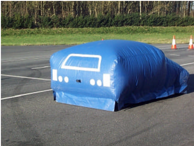
Figure 16. Inflatable car for testing system performance when colliding.
