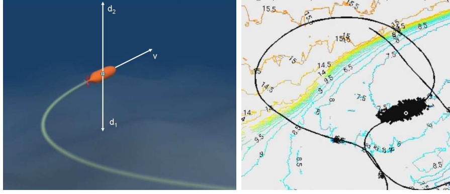
Fig. 13. The left plot is an illustration of an UW vessel measuring distance d_1 to sea bottom, and absolute depth d_2 . The sum d = d_1 + d_2 is compared to a bottom map as illustrated with the contours in the plot to the right. The particle cloud illustrates a snapshot of the PF from a known validation trajectory in a field trial, see [75].
