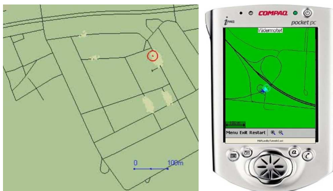
Fig. 15. Left: Example of multimodal posterior represented by a number of distinct particle clouds from NIRA Dynamics navigation system. This is caused by the regular road pattern and will be resolved after a sufficiently long sequence of turns. Right: PF in an embedded navigation solution runs in real-time on a pocket PC with a serial interface to the vehicle CAN data bus, see [80].
