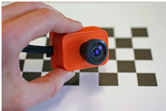
Figure 1: The sensor unit, consisting of an IMU and a spherical camera. The camera calibration pattern is visible in the background.
