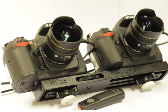
Figure 1: Stereo image registration hardware consisting of two 10 megapixel Nikon D200 DSLR cameras with Nikon 10.5mm f2.8 lenses and a common trigger.
