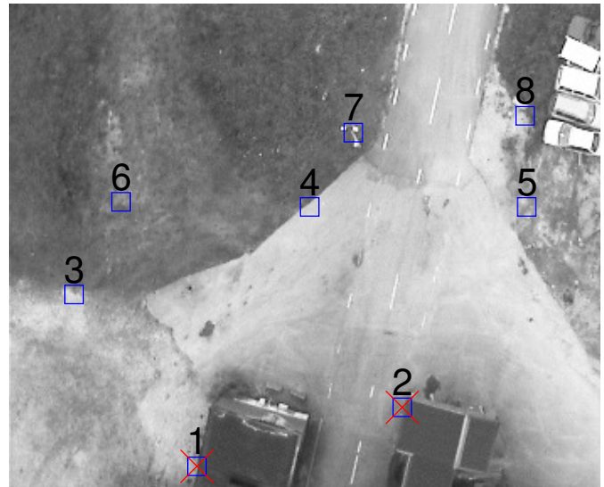
(b) Features detected in the second image, the group consisting of feature 1 and 2 are detected as inconsistent with the first image.
